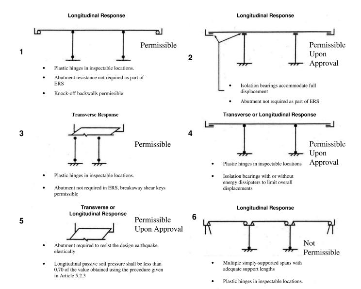
Figure 3.3-1a Permissible Earthquake Resisting Systems (ERS).
