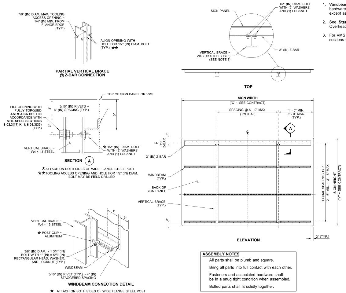
1. Windbeam and 3" (IN) Z-Bar are aluminum. All nuts, bolts, washers, and other hardware shall be stainless steel per **Standard Specification Section 9-28.11**, except as noted. Galvanize all non-stainless steel parts.
