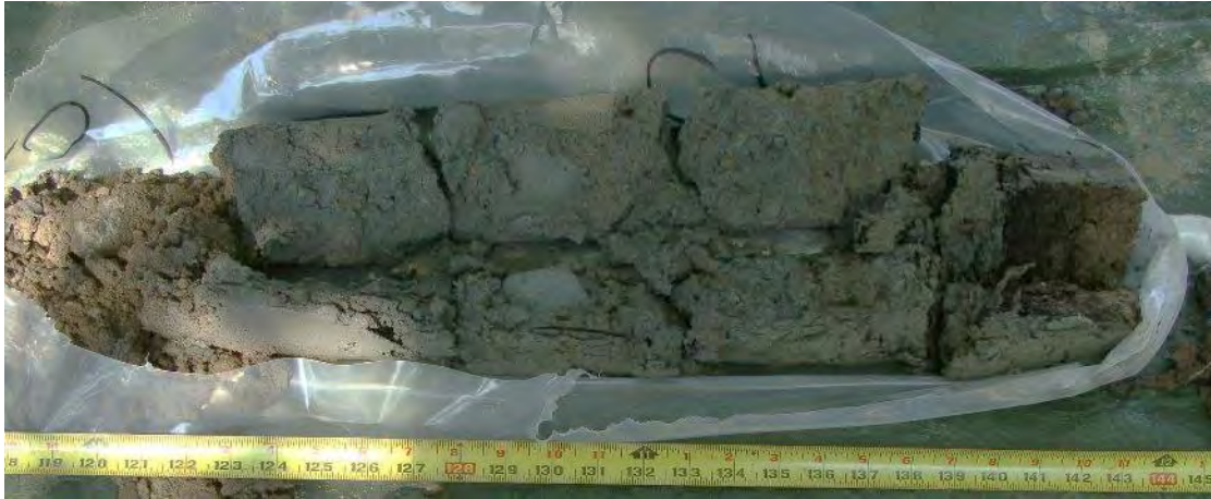
Figure 2-8. Example of a 6-inch-Diameter Sediment Sample Extruded into a Plastic Liner from a Rotasonic Sampler Tube. Note the presence of buried soil and subsoil at the downhole end of the sample on the right-hand side of the screen. This buried soil was identified approximately 12 feet below the ground surface.
