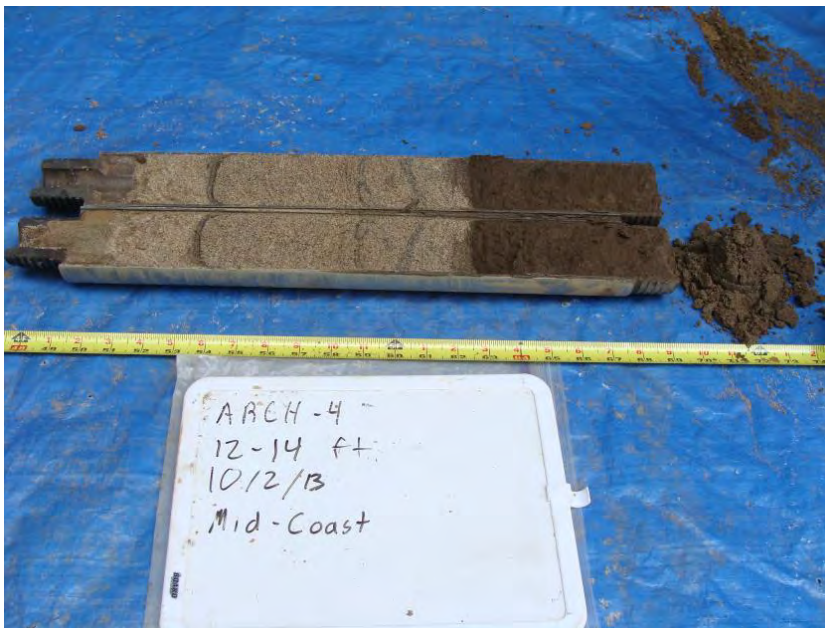
Figure 2-4. Example of a 4-inch Diameter Split-Spoon Sampler, Split Lengthwise with Bisected Sample Exposed
