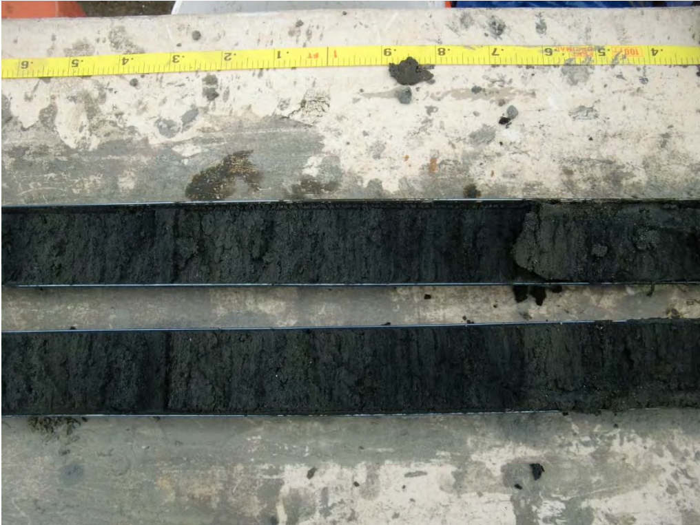
Figure 2-7. Example of a 2-inch-Diameter Sediment Sample Split Lengthwise in a Disposable Plastic Liner
